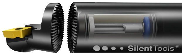
The dampening system consists of a heavy mass, supported on rubber spring elements
